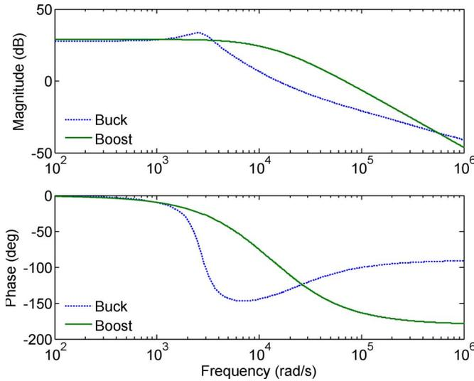
Fig. 13. Bode diagram of buck and boost topologies under nominal operating condition.
