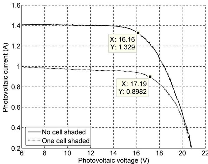
Fig. 2. Measured  $I-V$  curves of one-cell-shaded and nonshaded modules.
