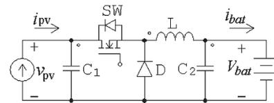
Fig. 11. Equivalent circuit of a buck dc/dc topology used as the photovoltaic power interface.
