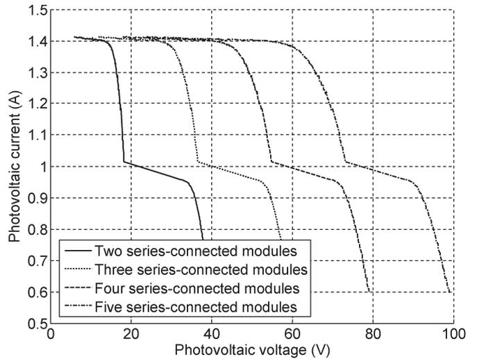
Fig. 3. Measured  $I-V$  curves when the one-cell-shaded module is series connected with the other nonshaded modules.
