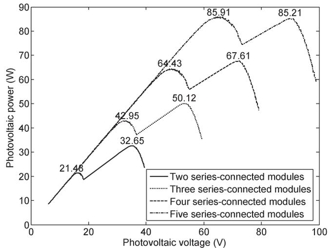
Fig. 4. Measured  $P-V$  curves when the one-cell-shaded module is serially connected to other nonshaded modules.
