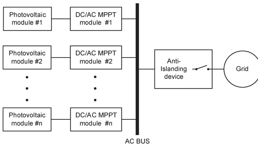
Fig. 16. Topology of grid-connected photovoltaic power systems with an ac bus configuration.
