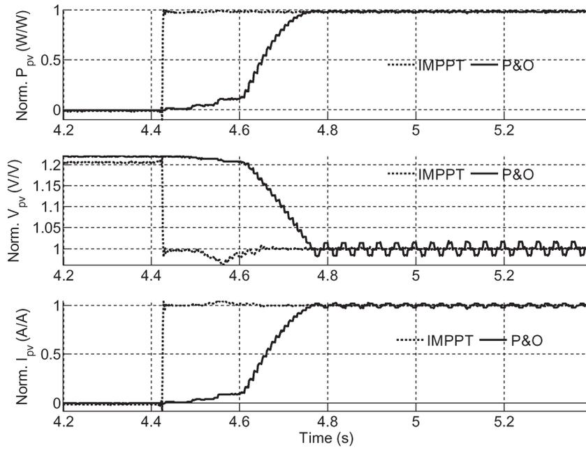
Fig. 9. Measured start of MPPT between IMPPT and P&O.
