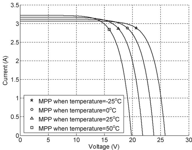
Fig. 7. Simulated  $I$ - $V$  curves of BP350 influenced by cell temperature when the insolation is constant  $1000\text{ W/m}^2$ .
