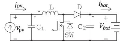
Fig. 12. Equivalent circuit of a boost dc/dc topology used as the photovoltaic power interface.
