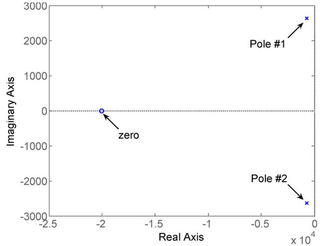
Fig. 14. Pole and zero locations of the system using buck topology.
