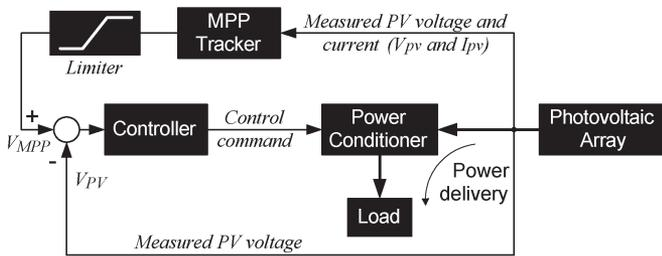
Fig. 10. Recommended control mechanism for MPPT.
