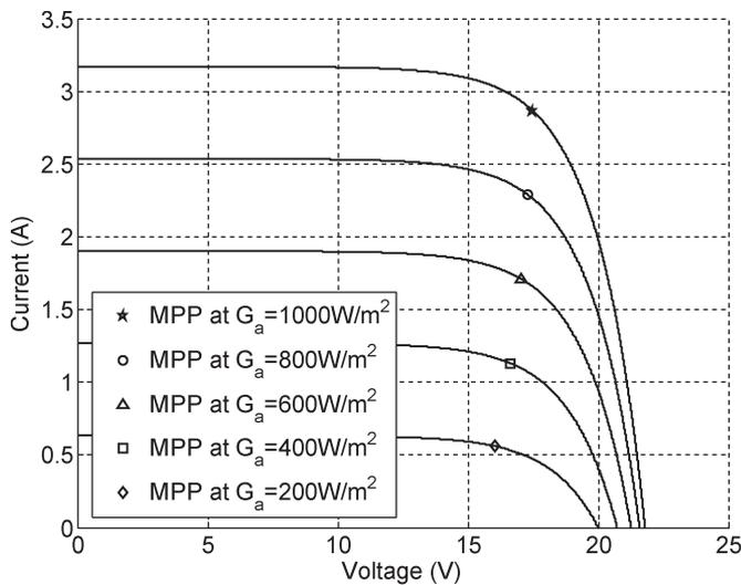
Fig. 6. Simulated  $I$ - $V$  curves of BP350 influenced by insolation when the cell temperature is constant  $25\text{ }^\circ\text{C}$ .
