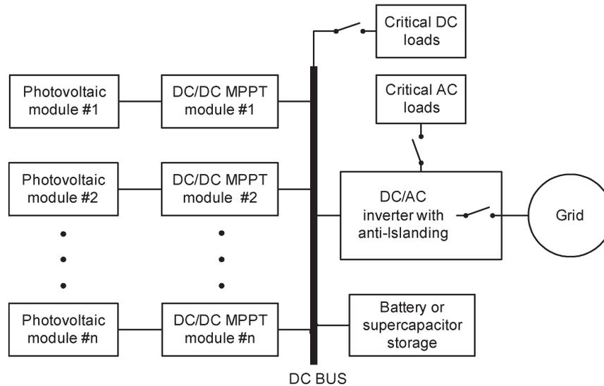
Fig. 5. Topology of grid-connected photovoltaic power systems with a dc bus and a UPS function.
