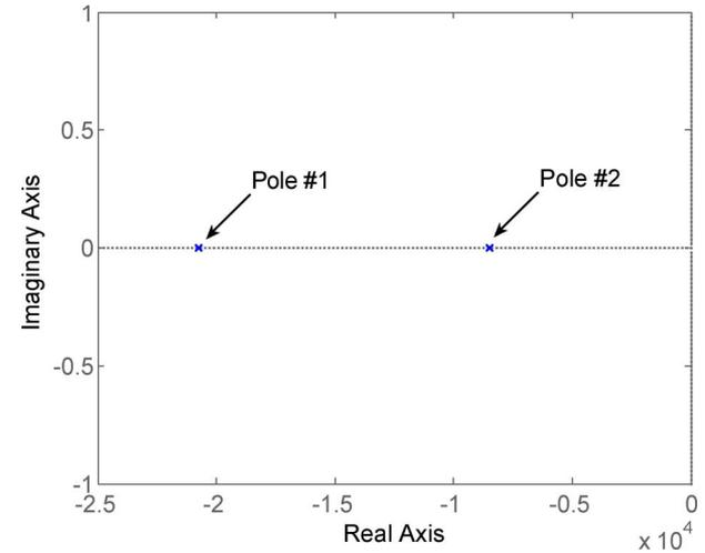
Fig. 15. Pole locations of the system having boost topology.
