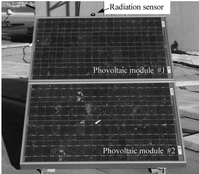
Fig. 1. Two photovoltaic modules installed on one frame at the same angle and direction.
