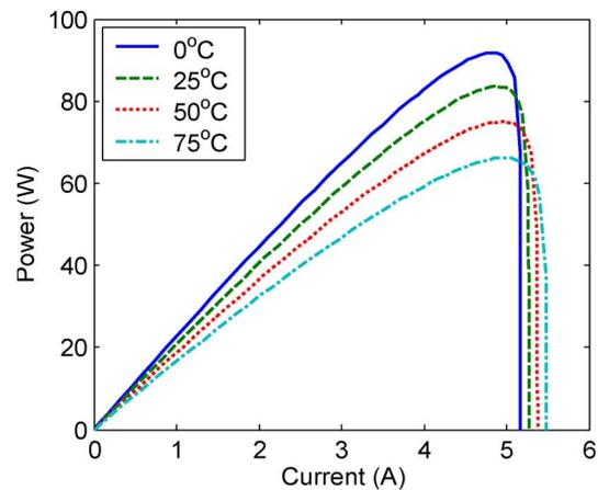
Fig. 8. Temperature effect on the relationship of power and current of MSX-83 solar panel with a constant insolation equal to  $1000\text{ W/m}^2$ .
